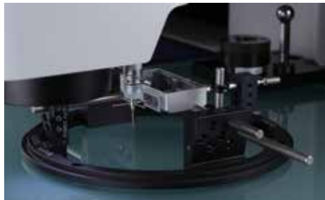
QV Active with optional Opti-fix clamping system
