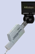
SurfTest Probe (surface finish)
