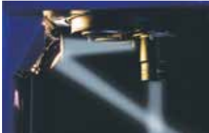
Switchable surface illumination: vertical or oblique
