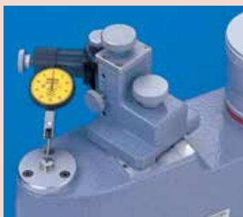
Calibrating test indicator
